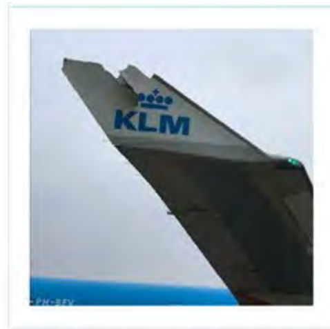
Figure 3b: Damage to the B747's right wingtip. (Source: Amsterdam Airport Schiphol)
