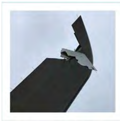
Figure 3a: Damage to the B787's right horizontal stabiliser. (Source: Amsterdam Airport Schiphol)
